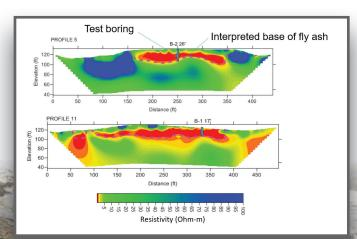
Electrical resistivity profiles were paired with geotechnical boring logs to interpret the thickness of fly ash.
