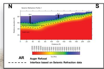
Boundaries of soils, partially weathered rock and unweathered rock captured by refraction seismics. Geophysical profiles were correlated with geotechnical borings to provide the client with a comprehensive understanding of the site.
