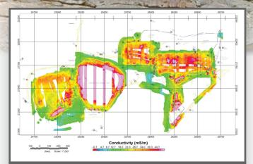
Example of an electromagnetic contour map of landfill boundaries. Oranges to reds indicating areas of conductive soils (landfill) and metallic buried objects.
